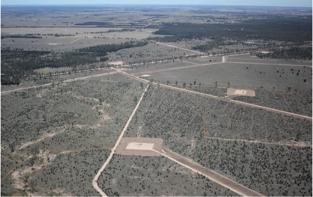
Fig. 19.10. The patchwork of CSG wells near Chinchilla in Queensland, showing the potential network of roads and cleared platforms that may serious affect river flows of the Lake Eyre Basin if established in the Channel Country (photo, R. T. Kingsford).
